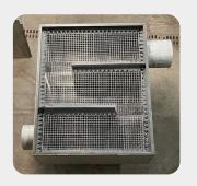
In 2024, our team mitigated this noise by designing an insulated damper box that essentially worked as a silencer, which reduced the noise from 95 decibels – comparable to the sound of a typical chainsaw – to a more comfortable ambient level of 55 decibels, similar to a household fan. This substantial improvement created a safer and significantly less noisy working environment for our associates and considerably lessened noise disturbance for the local community.
